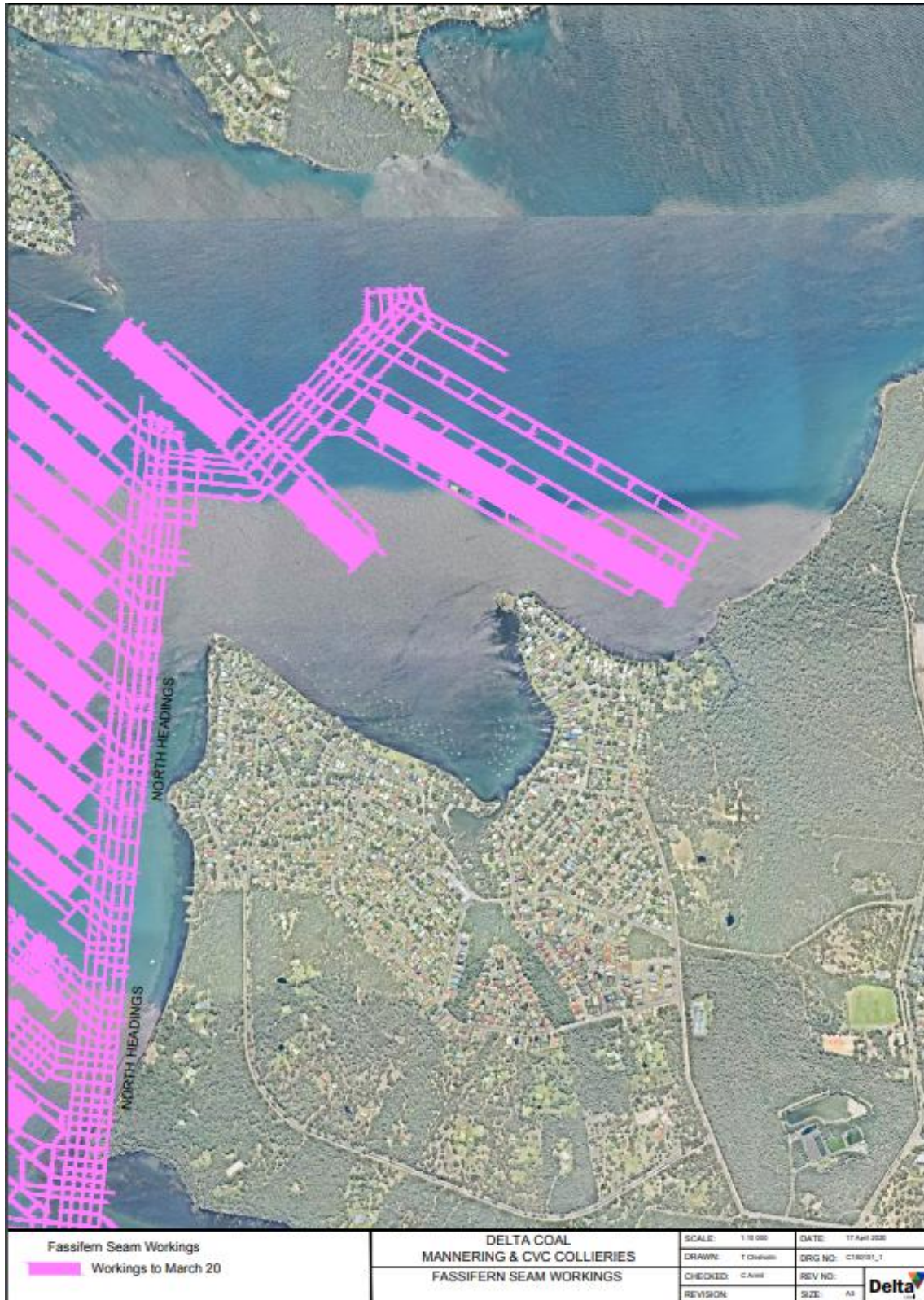
Figure 10.1 Extent of Fassifern seam workings to March 2020.
